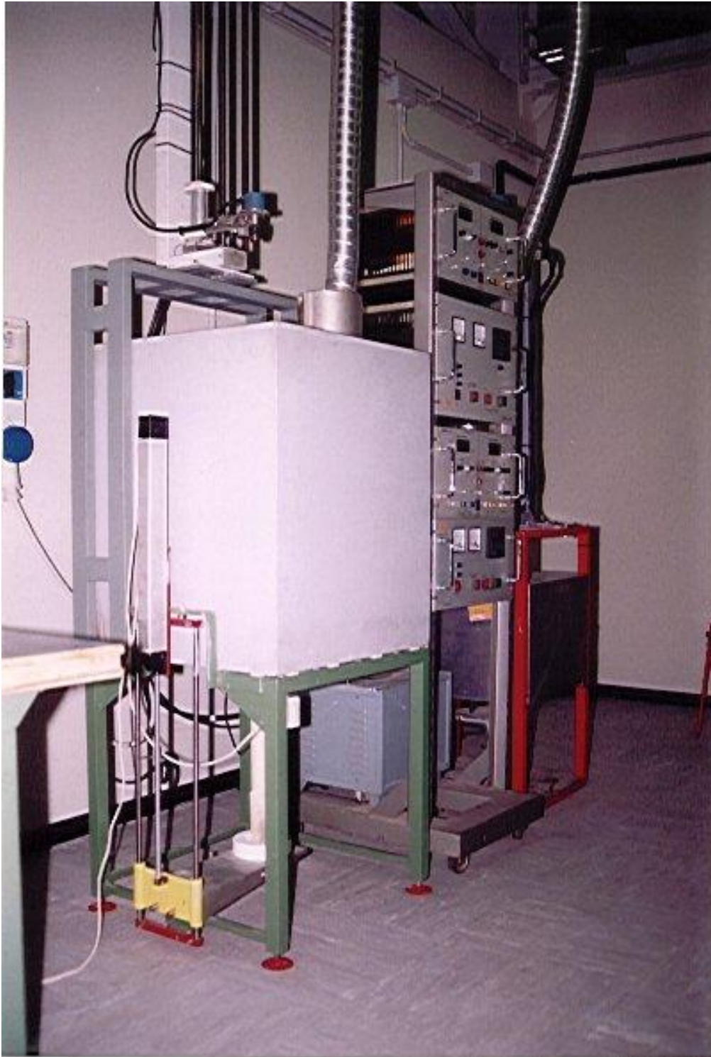
Furnace for epitaxial growth of garnet films
