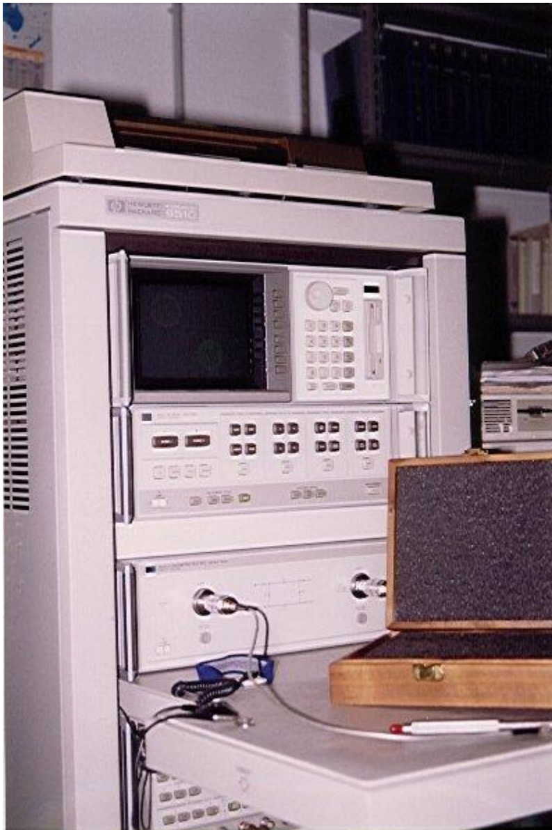
Two HP8510C Vector Network Analyzer for S-parameter measurements: (i) up to 18 GHz and (ii) up to 50 GHz
