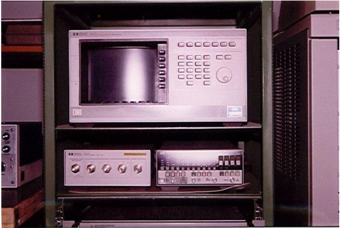
HP digital oscilloscope for microwave and optical devices characterization up to 20 GHz
